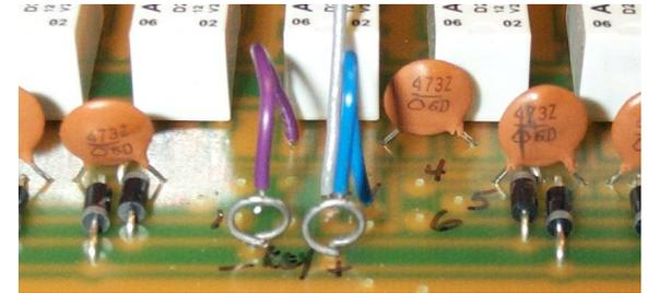
terminal in NEGATIVE mode. It is used to provide Back EMF suppression across the relay solenoids. This protects interface devices from possible spikes. It is not strictly required for use with mechanical switching.
